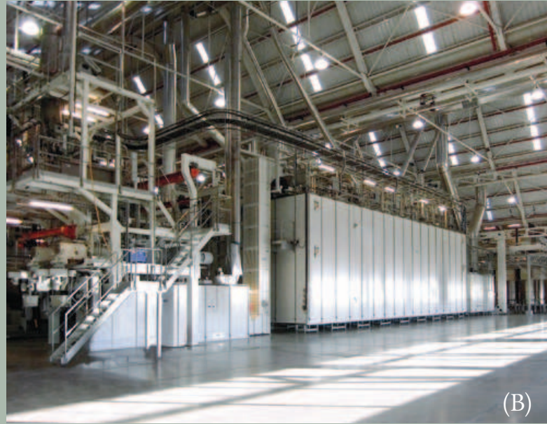
Two lines for long (A) and short-cut (B) pasta production recently developed by Fava.
